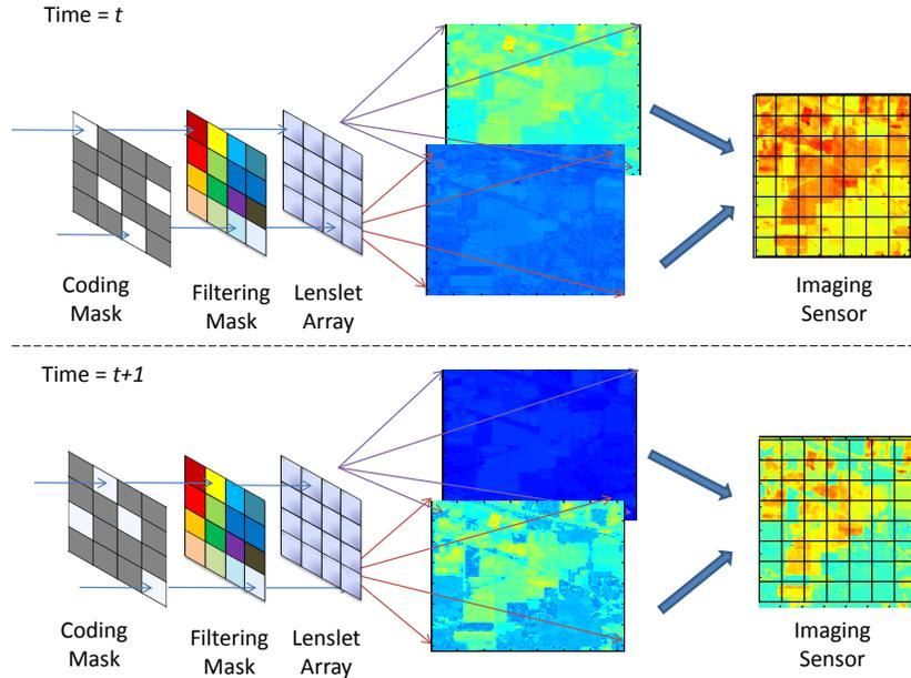
Figure 1: Image acquisition via the proposed scheme in two different sampling instances. During each sampling instance, the pattern of the coding mask allows the propagation of light from a specific spectral band which is optically multiplexed in the imaging sensor.
